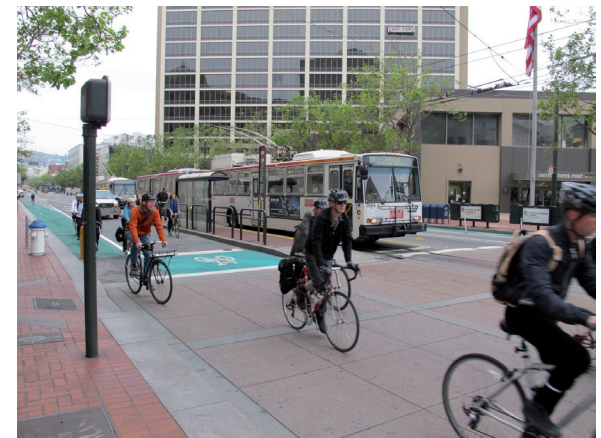
Recent efforts to allocate space and improve safety for bicycles are illustrated here with painted bike lanes and a "bike box" which serves as a waiting area for bikes.
