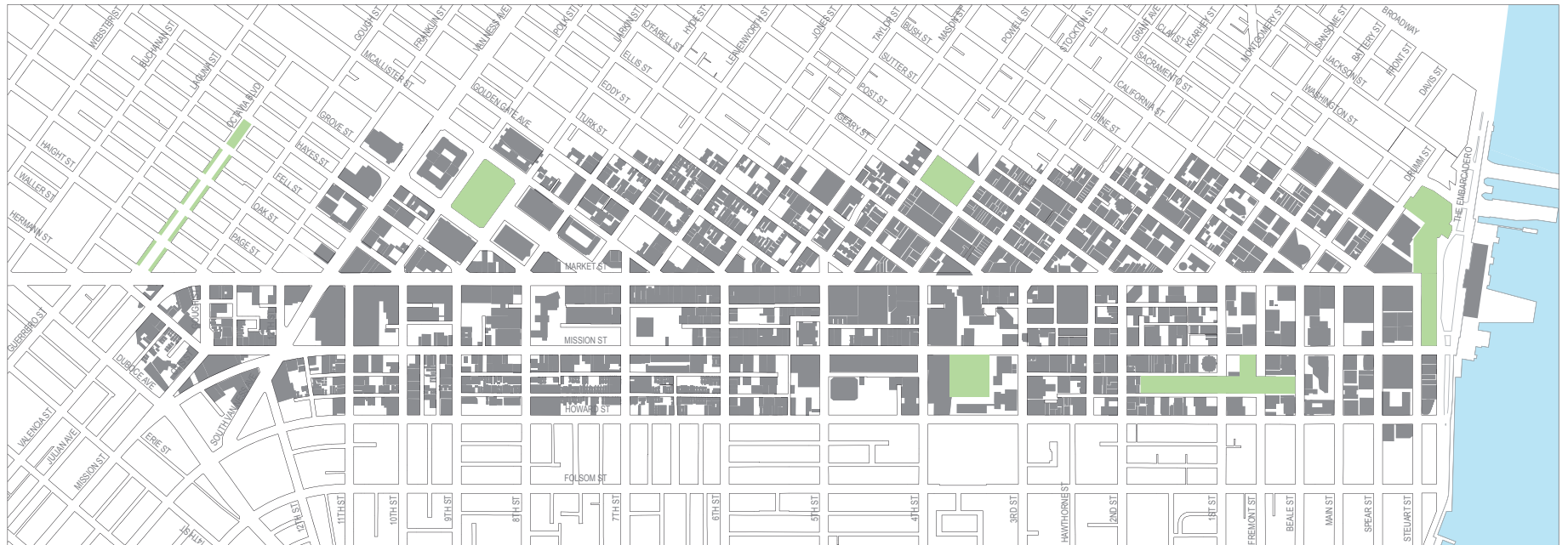
Fig. L - This “figure ground” diagram illustrates the pattern of building footprints on the blocks lining Market Street. Clearly apparent are the differences in block size north and south of Market Street and the scale of buildings that exist on those blocks. Uninterrupted facades, especially along the south side result in uncomfortable long walks for pedestrians and few places to cross the street.
