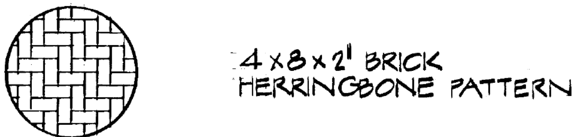
Figure 1-5. From Contract Drawings for Market Street Reconstruction: Herringbone Brick Pattern
