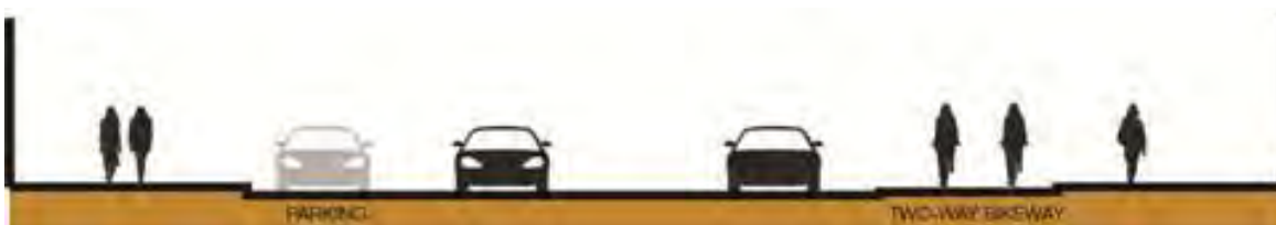
Figure 8. Mission Street Bikeway with Two-way Cycle Track on One Side. Parking strips are 8 feet wide, travel lanes for vehicles are 12 feet wide, and the bikeway is 16 feet wide with a 4.5-foot buffer.
