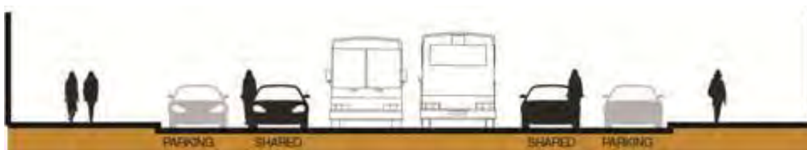
Figure 6. Mission Street Alternative with Center-running Bus Lanes. Bus lanes would be 13 feet wide, the outer lanes would be 13 feet, 3 inches wide. The illustration shows the condition outside of the Sixth Street to Fremont Street corridor (within which there would be no space for parking).
