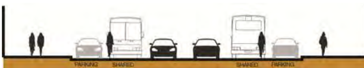
Figure 7. Mission Street Alternative with Side-running Bus Lane. Inner traffic lanes would be 9 feet wide; outer transit lanes with parking would be 17 feet, 3 inches wide.
