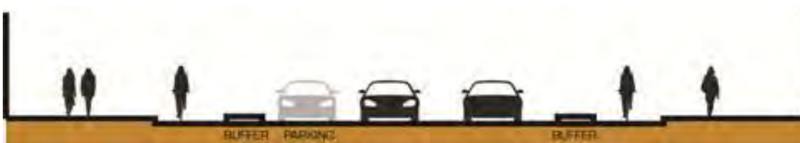
Figure 9. Mission Street Bikeway with One-way Cycle Track on Each Side. Bikeways are 6 feet wide, buffers are 4.5 feet wide, floating parking strip is 8 feet wide, and travel lanes are 12 feet wide.
